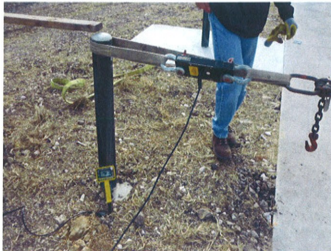
Figure 8 URBS Bollard Prior to Testing
