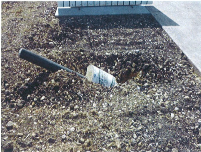
Figure 5 URB-1 Bollard Following Testing
